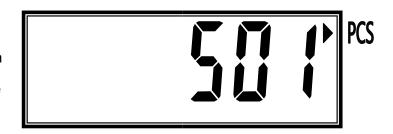
• Press FUNCTION key to exit simple counting mode and move back to weighing mode.
